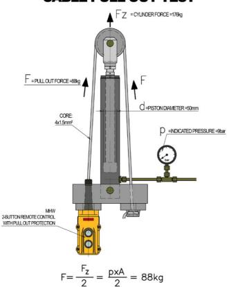
A specially designed "Pull-Out-Protection" eliminates contacts from being torn out, causing electrical shorts.
